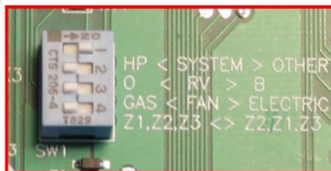
Figure 10: Factory Dip Switch Setting Closeup
