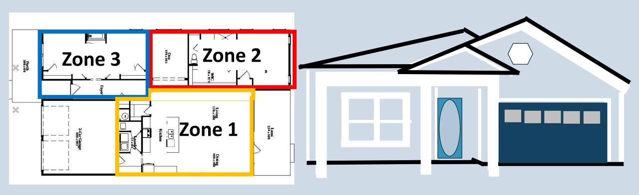
Three thermostats + three zones + full HVAC system airflow capacity to one zone at a time = comfort control for diversity!
